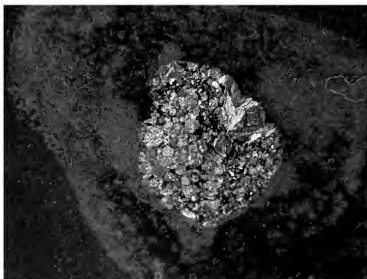
Fig.15- Transmitted crossed polarized light photomicrographs showing zoning olivine crystal. The zoned color range from the crystal's rims to the center of the crystal is an indication of zoning characterized by the change in the mineral composition. Length of field 0.45mm.
